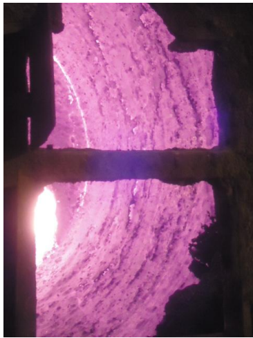
Fig. 4: MAC bricks with CaO-MgO-Al 2 O 3 aggregate after 10 heats in a 205 steel ladle in an integrated steel shop.
