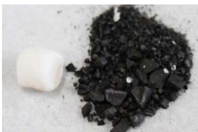
Fig. 7 Crushed MgO pellet after the reduction test.
