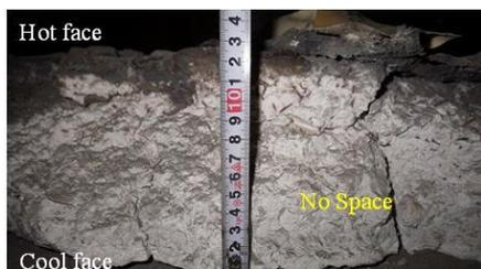
Figure 10. Cross section of the Case 2 impact pad after actual
