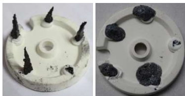
Fig. 5: Cones before and after the critical temperatures determination.
