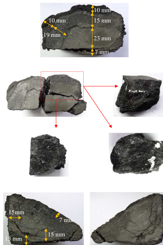
Fig. 2: Internal aspect of the post mortem \text{SiC} bricks.
