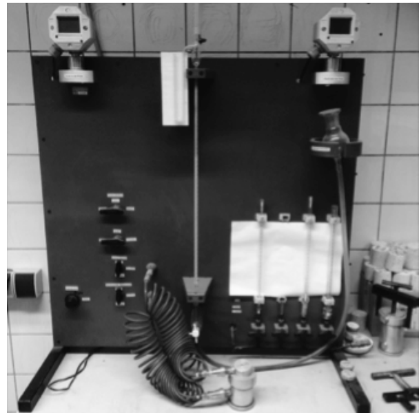
Fig. 2: Permeability measurement device according to DIN EN 993-4
