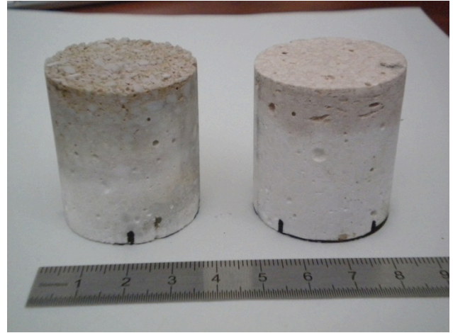
Fig. 5: Corroded samples with 15 g of waste slag (left) and 5 g of steel slag (right). 1550 °C for 70 hrs.
