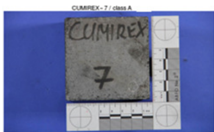
Fig.8: Nitride bonded SiC sample after CO disintegration test
