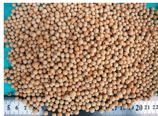
Fig. 6: Mullite based hollow balls sized 3-5mm
