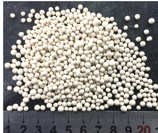
Fig. 9: Synthesized porous forsterite balls with sizes 2-5mm
