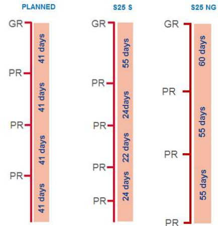
Fig.7. Comparison between planned trough campaign and actual ones with S25 S or S25 NG. GR: General repair; PR: Partial repair.
