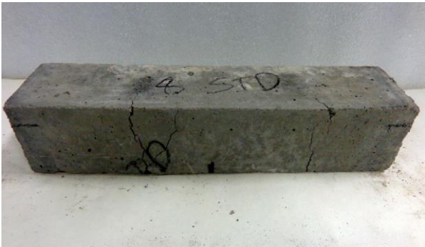
Fig. 7: Conventional cast bar, after 100 hour CO disintegration test
