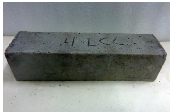
Fig. 4: LCC cast bar, pre-CO disintegration test
