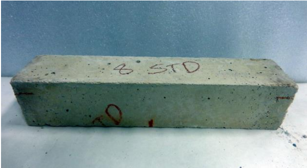
Fig. 6: Conventional cast bar, pre-CO disintegration test
