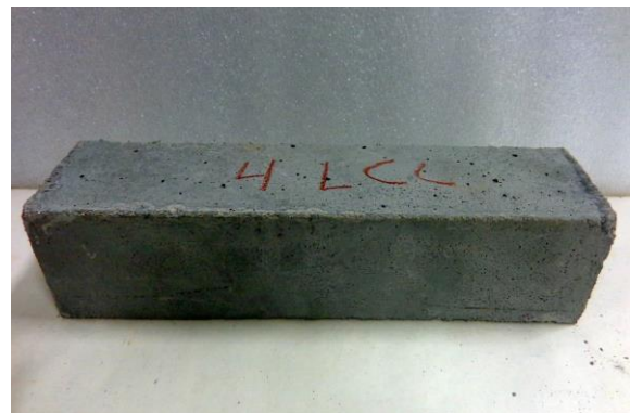
Fig. 5: LCC cast bar, after 100 hour CO disintegration test
