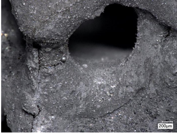
Figure 1: Optical micrograph of the filter surface after 10 s of contact with the steel melt.
