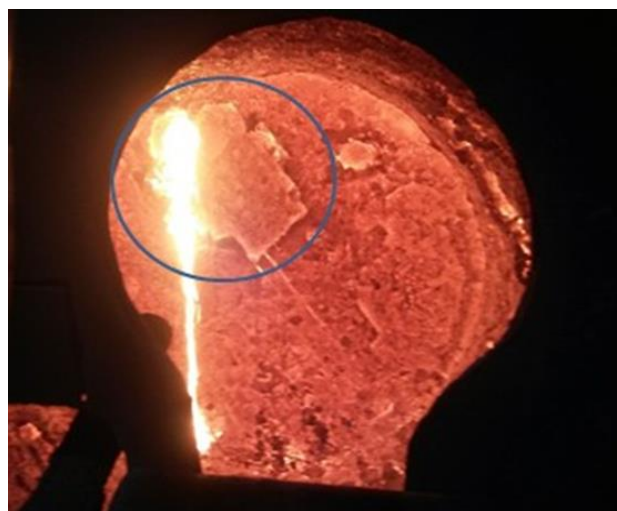
Fig. 2 - Steel ladle bottom after 72 heats, showing spalling of bricks at region between well blocks.
