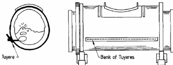
Fig. 1: Schematic of a Pierce-Smith Converter.<sup>[1]</sup>
