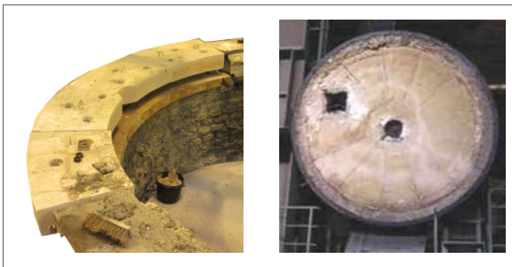
Figure 7: Left: upper block for steel ladle Right: Ladle preheater cover
