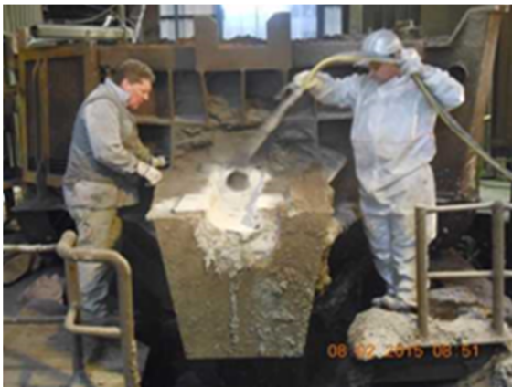
Figure.11: Cold and hot repair in an EAF
