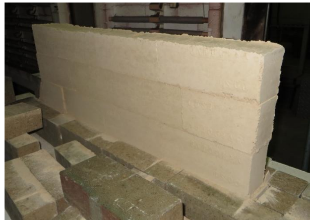
Fig. 7: Simulated permanent lining with dry setting mix fired at 1000 °C.
