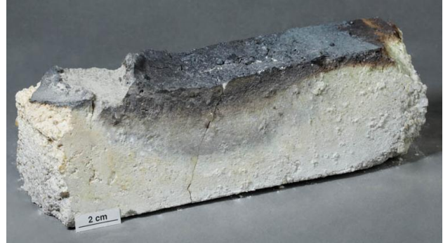
Fig. 10: Cut segment of dry setting mix from IF test.
