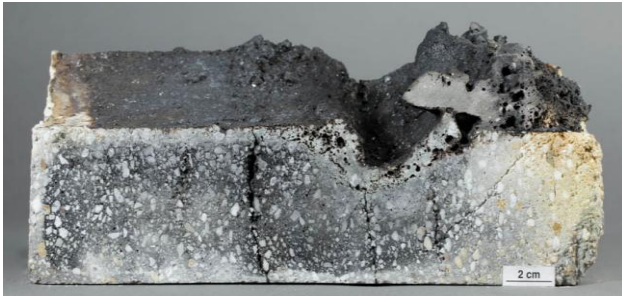
Fig. 8: Cut segment of ready-for-use mix with additives from IF test.
