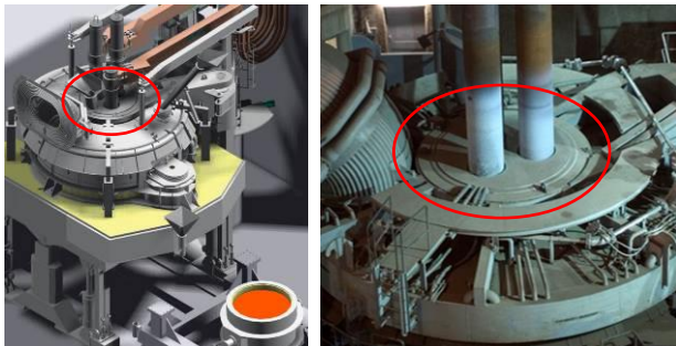
Fig. 1: EAF design [1]- delta roof red circled.
