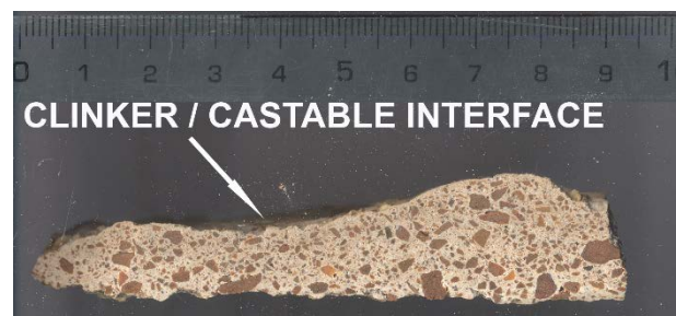
Fig. 9: Cross section of Magnesia-Spinel castable after 5 day of operation.
