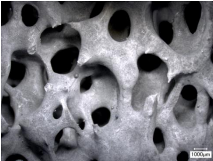
Figure 3: Overview of the CA6-C filter surface after 10 s of contact with the steel melt.
