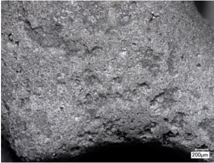
Figure 2: Detail of the CA2-C filter surface after 10 s of contact with the steel melt.
