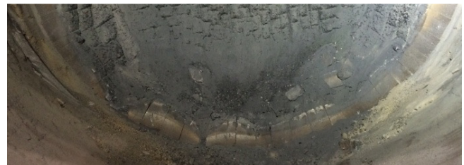
Fig. 7: Wrecking of a standard tuyere zone
