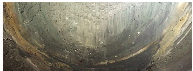
Fig. 8: Wrecking of a fused doloma containing tuyere zone (same AOD and location)
