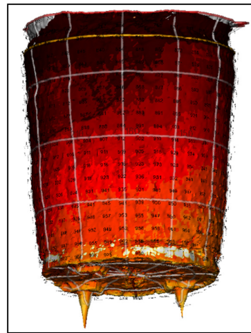
Fig. 6 Temperature Profile of ladle bottom and wall
